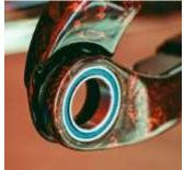
SRAM has also designed in some new features! It uses the thru axle as its mount rather than having a separate mount, it swivels on a bearing thereby allow some movement if it is struck, and it has a hook shape on top to stop the chain from becoming wedged between the frame and Freehub body (chain suck).
